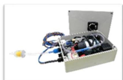
The pump should hardly need to run. If it does, then check that all the vacuum connections are good, and the end tails are on their dollies. The vacuum high limit is set by a switch mounted within the pump.
