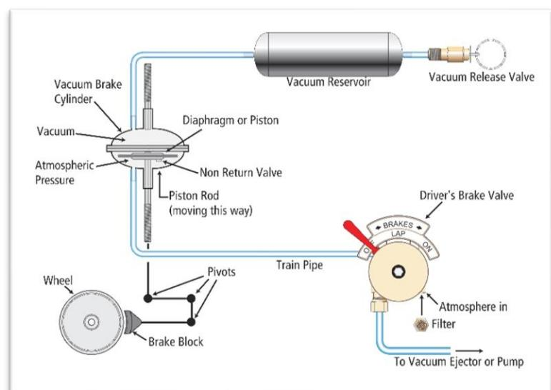
The vacuum is trapped on the upper side of the diaphragm by the non-return valve. The vacuum must be re-created in the train pipe to release the brakes.
